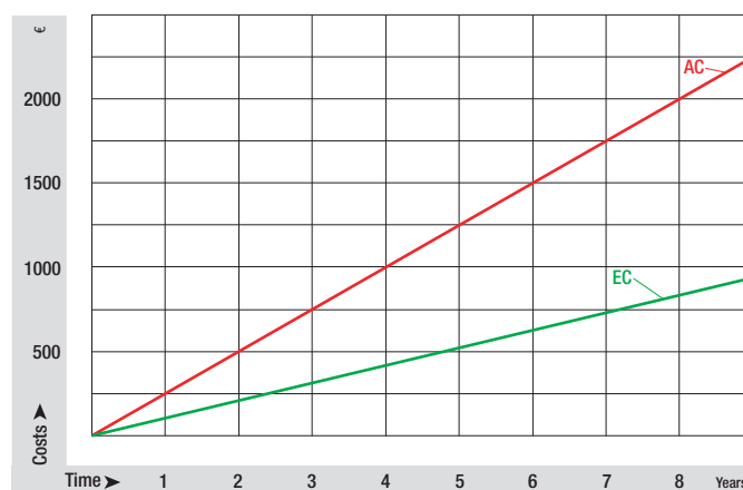
Figure: Operating costs over time at 0.10 EUR/kWh
